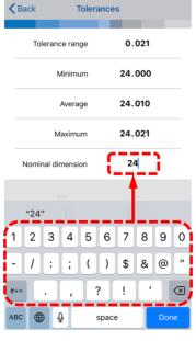
Enter the nominal dimension of the workpiece (Click in the input box to display the keypad)
